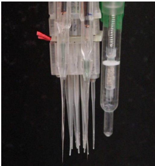
Disposable ion-selective membrane sensors (center), oxygen microsensor (left) and reference electrode (right) for in-situ measurements in soft sediments (Martin Maerki).
