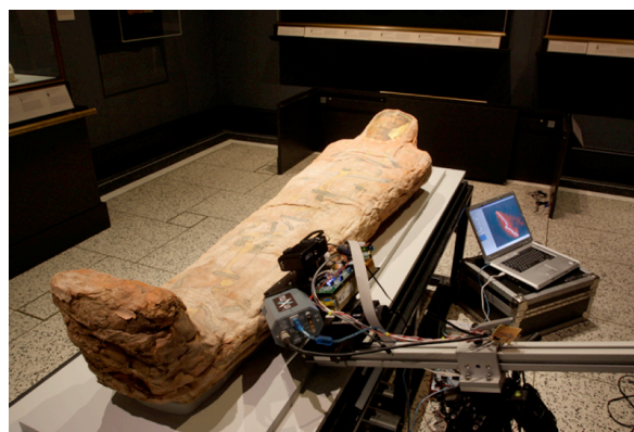
Figure 13. Duetto Instrument with Mummy. Duetto, commissioned by the Getty Conservation Institute, is a commercial spinoff of CheMin, is used for in situ art characterization and art conservation.
