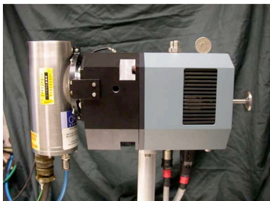
Figure 2 (b). CheMin II instrument. The instrument consisted of an Andor™ CCD camera interfaced to a sample chamber (kept at atmospheric pressure), bolted to an Oxford X-ray Technology Group micro-focus X-ray tube. The detector is an E2V 5530 1250 X 1150 pixel CCD imager. Samples could be exchanged in air, without disturbing the alignment of the instrument. Power supplies for the X-ray tube and camera are not shown. The instrument is air cooled.
