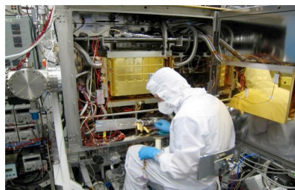
Figure 9. The SAM suite is here being prepared for tests in its environmental chamber that span the range of temperatures and pressures that SAM will encounter on the surface of Mars.
