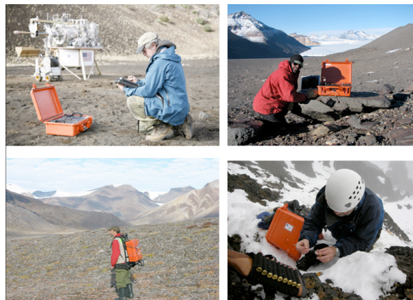
Figure 8. Use of Terra during NASA and other field campaigns. (a) The author (NASA/ARC) during the Scarab/RESOLVE field test on Mauna Kea, HI (2008). Terra was used to analyze as-received volcanic soils and partial run products from In Situ Resource Utilization (ISRU) experiments. Lunar oxygen-generating equipment in the background. (b) Doug Ming (NASA/JSC) on an expedition to the dry valleys of Antarctica (2008). Terra was used to analyze soils and other materials to understand pedogenesis (soil generation) in cold, dry climates. (c) Ron Peterson (Canadian Geological Survey), in the high Arctic of Canada (2009). Searching for low-temperature stability minerals such as the hydrates of iron and magnesium sulfate. (d) The author (NASA/ARC) during the AMASE expedition in Svalbard, Norway (2009). Analyzing carbonate sediments and cements in volcanic vents for clues as to their origin.
