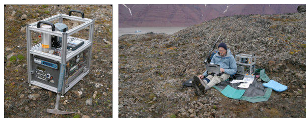
Figure 2 (d). CheMin IV. (left) As deployed in Svalbard, Norway in 2006. (right) CheMin Co-I Dave Bish of Indiana University performs the first complete XRD/XRF data collection and quantitative analysis in the field. The instrument is fully self-contained, operated with an integrated computer and on-board lithium batteries and power supplies. Once an analysis is completed, the raw data are downloaded onto a USB storage drive and transferred to a laptop computer for processing.
