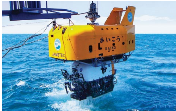
Figure 8. Launching the Japanese submersible KAIKO 7000 operated by JAMSTEC. Photograph provided by JAMSTEC.
