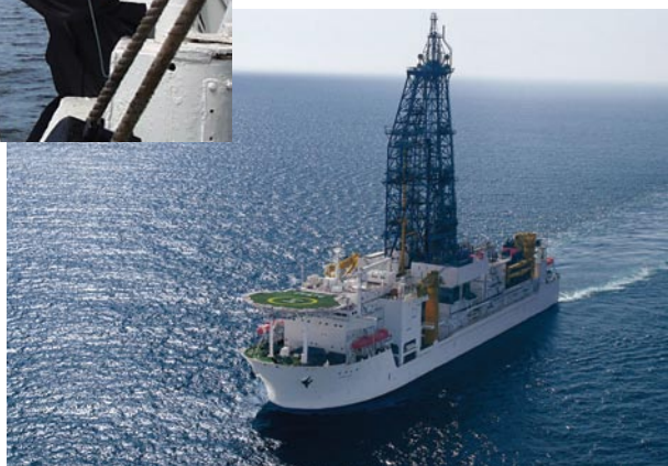
Figure 9. Left. Water sampling on Lake Baikal. Photo provided by Jens Klump. Bottom. Photograph of the Japanese riser drilling platform Chikyu , which is capable of drilling to 7000 m beneath the seafloor. Photo provided by JAMSTEC.
