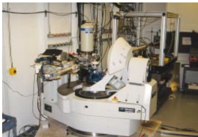
Diffractometer (foreground) and x-ray fluorescence microprobe (background) in experimental station 13-ID-C on the undulator beamline at GeoSoilEnviroCARS
