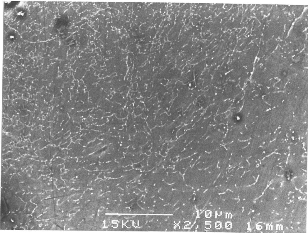
FIG. 2. Photograph of SEM backscatter image, showing small elongate bodies of magnesioferrite with high backscatter intensity in darker fPer matrix (specimen BZ70); scale bar 10µm.
